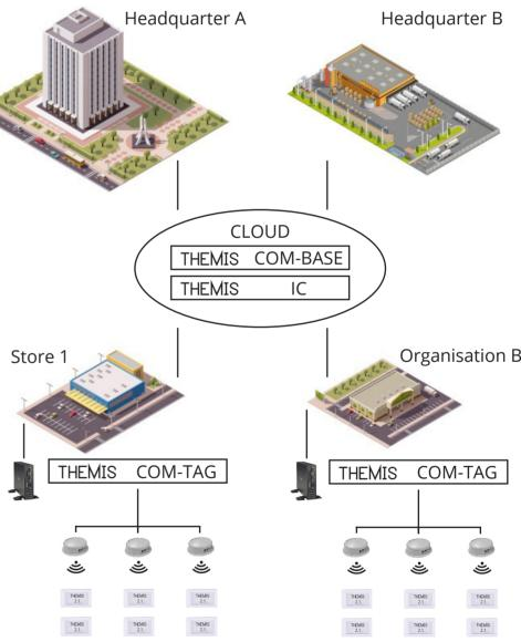
**CLOUD LEVEL** In this scenario, the COM-BASE and IC are installed in a cloud. Headquarters and branches communicates directly through a cloud.
